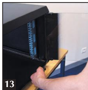
13 Check the door for squareness and lock it into position.
